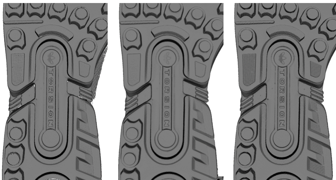
Figure 100: Models of a shoe sole obtained using various algorithms: Fast fusion (left), Smooth fusion (middle) and Sharp fusion (right).
