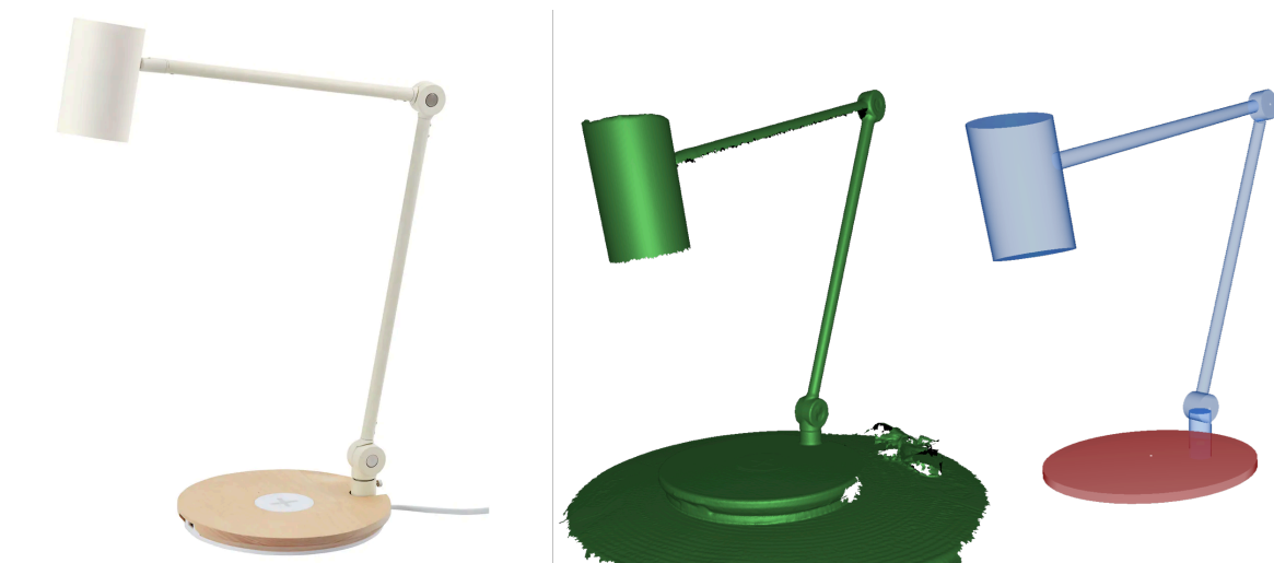
Figure 133: From left to right: original object, scanned model, a set of constructed primitives.
