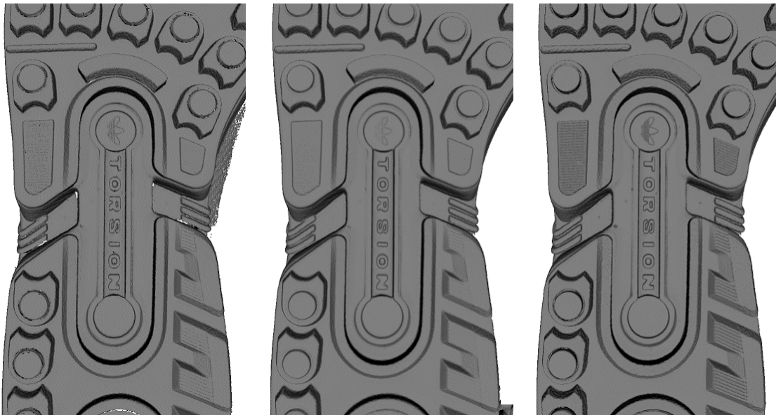
Figure 126: Models of a shoe sole obtained using various algorithms: Fast fusion (left), Smart fusion (smooth, middle) and Smart fusion (sharp, right).
