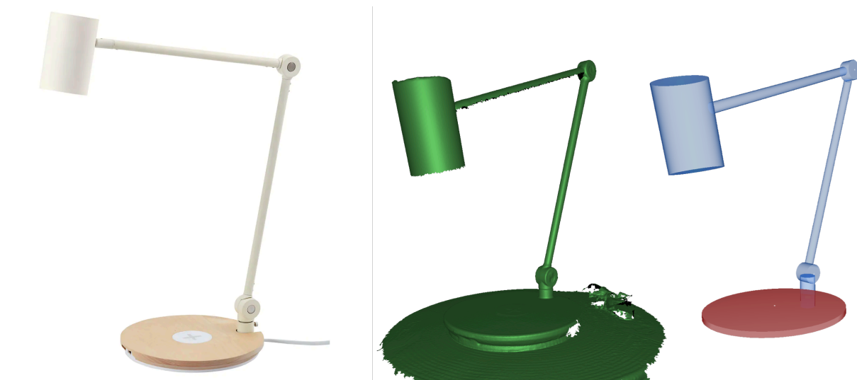
Figure 160: From left to right: original object, scanned model, a set of constructed primitives.
