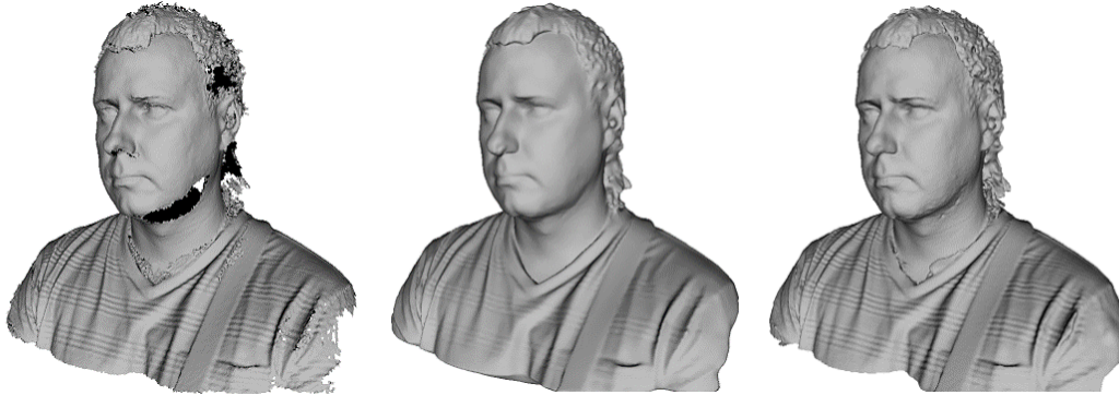
Figure 125: Models of a human subject obtained using various algorithms: Fast fusion (left), Smart fusion (smooth, middle) and Smart fusion (sharp, right).
