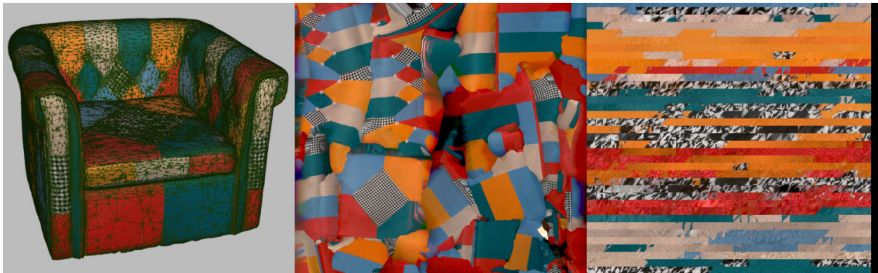
Figure 147: Texture mapping methods: mesh with texture applied (left), texture-atlas sample (middle) and triangle-map sample (right). The latter covers only a portion of the mesh surface (the rest two images not shown).
