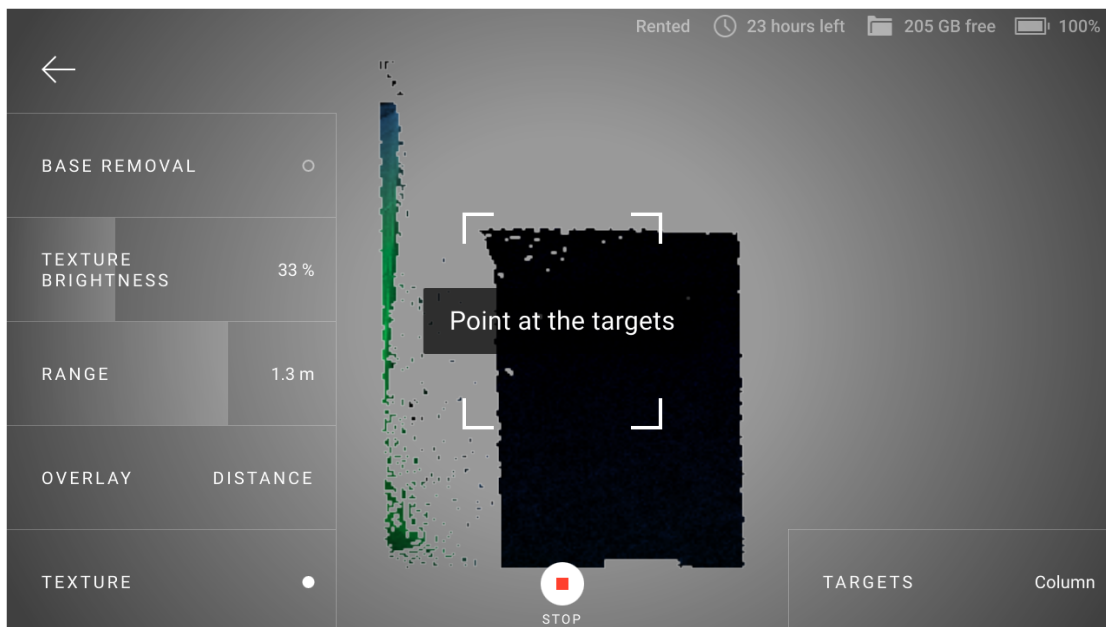
Figure 10: Target-assisted scanning mode is set but Leo does not see targets in its field of view.
