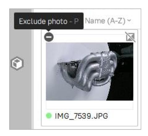
If a mask includes a stand or part of the object that extends beyond the cropping box, it can potentially lead to artifacts after **Create Model**. In this case, try expanding the cropping box to encompass both the object and the stand entirely.
