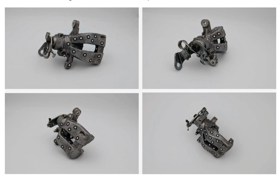
2. Adjust target size by expanding the **Advanced** section on the **Scan** panel in Artec Studio.
