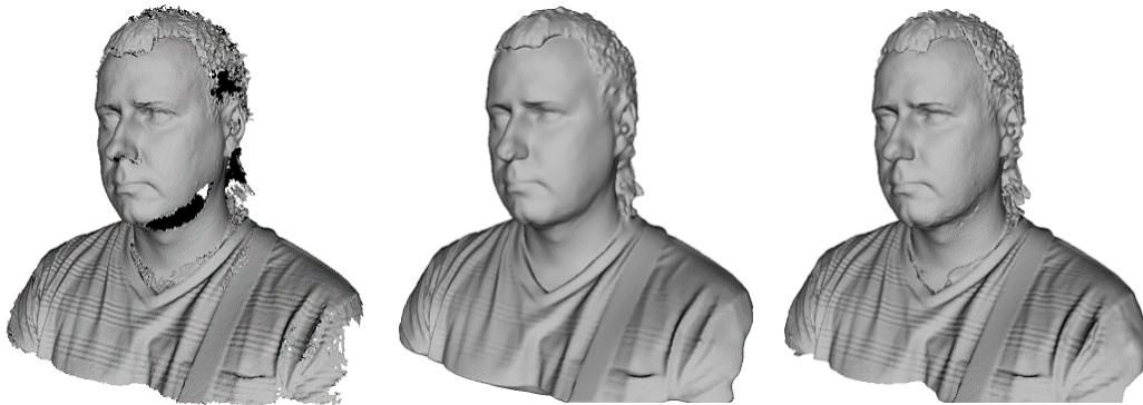
Figure 137: Models of a human subject obtained using various algorithms: Fast fusion (left), Smart fusion (smooth, middle) and Smart fusion (sharp, right).
