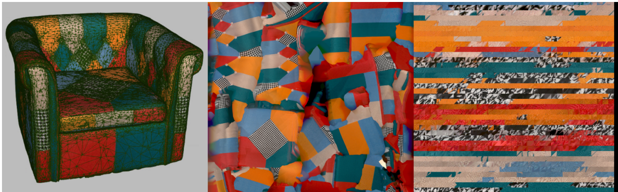
Figure 161: Texture mapping methods: mesh with texture applied (left), texture-atlas sample (middle) and triangle-map sample (right). The latter covers only a portion of the mesh surface (the rest two images not shown).
