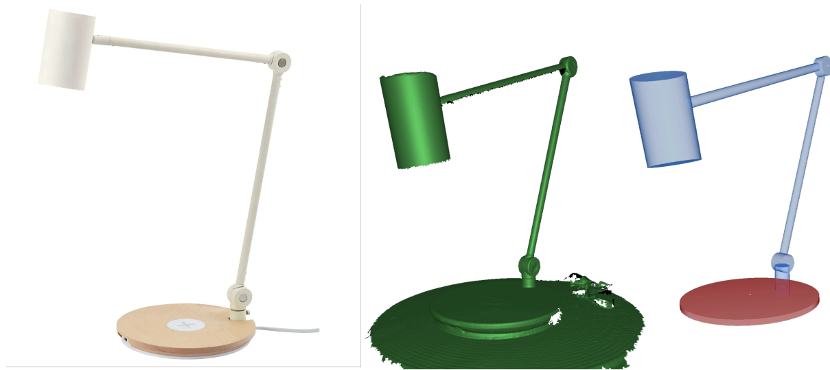
Figure 174: From left to right: original object, scanned model, a set of constructed primitives.
