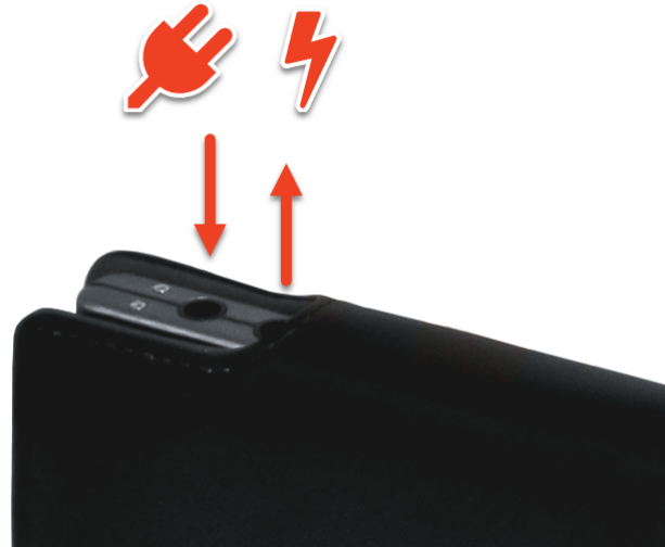
Figure 27: Battery ports from left to right: Input, Output.
